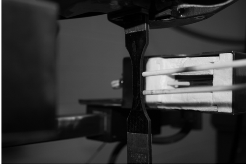
Figure 18 MTS High temperature axial extensometer attached to test specimen
