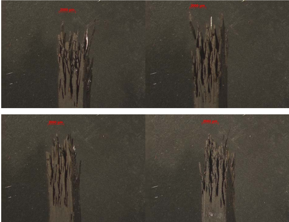
Figure 51 Carbon fiber reinforced PMR-15 composite specimen 2 aged in argon for 100 hours at 288°C (side view).
