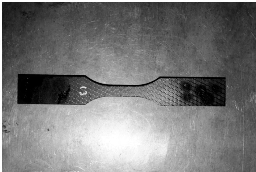
Figure 13 Test specimen before tabbing
